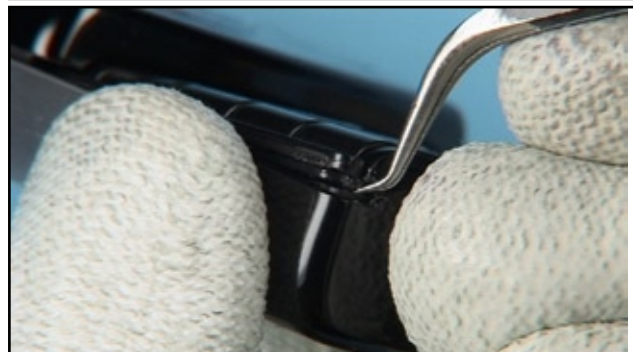
24. Locate the small recesses. shift the clip of the BOTTOM KEYMAT outside.
